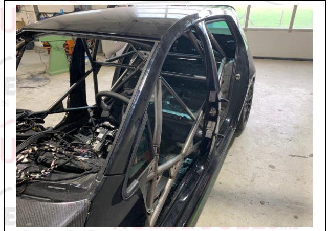
PHOTO 2 REAR ¾ VIEW OF CAGE
