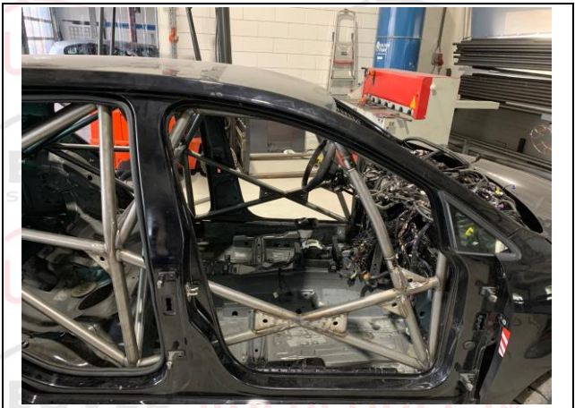
PHOTO 11 ANTI-INTRUSION DOORBAR – CO-DRIVER
