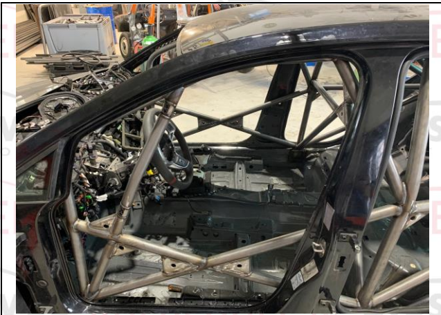
PHOTO 10 ANTI-INTRUSION DOORBAR - DRIVER
